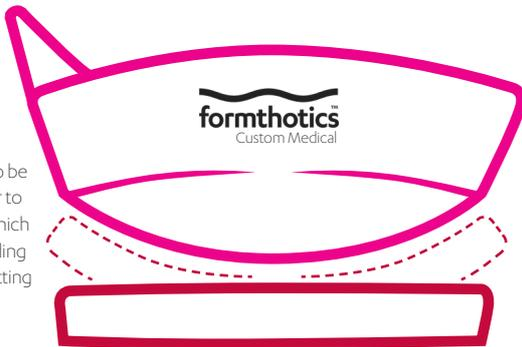
Additions need to be "cupped" in order to adhere to base which may require grinding to allow proper fitting into footwear
