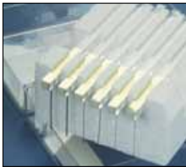
Figure 1. An original three-force set of monofilaments. Two each of 4.17/1g, 5.07/10g and 6.10/75g.
