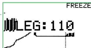
6. Press LEG/TOE button to save the ankle pressure.
