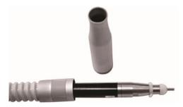
Fig.12: Removing the handpiece cover
