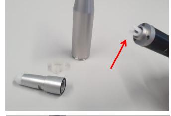
6. Secure the new collet with a 10 mm open-end spanner in a clockwise direction.
