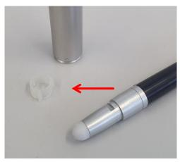
3. Loosen and remove the collet with a 10 mm openend spanner by turning it anticlockwise.
