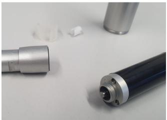
5. Insert the new driver. Place the flat surface onto the motor shaft. Ensure that the driver is positioned correctly. Otherwise, it may be damaged.
